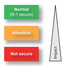
**Green** means that an outage of one element will not cause an overload. **Yellow** means that one or morebranches exceed the first loading threshold. Moreo-
